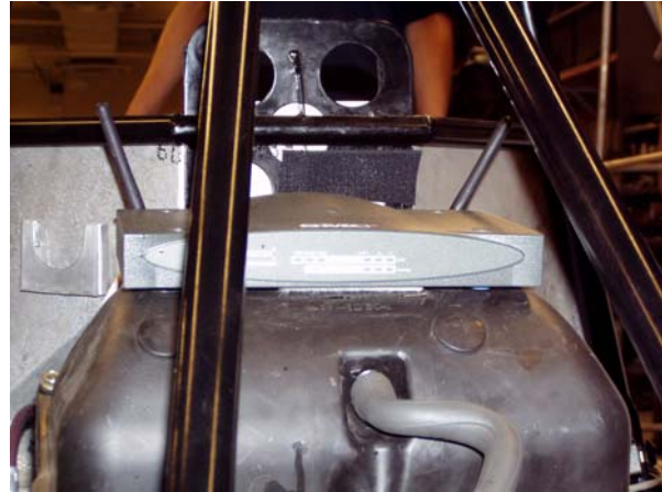
Rear view of a DATAQ Instruments DI-720EN mounted inside one of the cars (left) and the SMC wireless access point mounted atop the engine (right).
