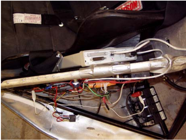
Rear view of a DATAQ Instruments DI-720EN mounted inside one of the cars (left) and the SMC wireless access point mounted atop the engine (right).
