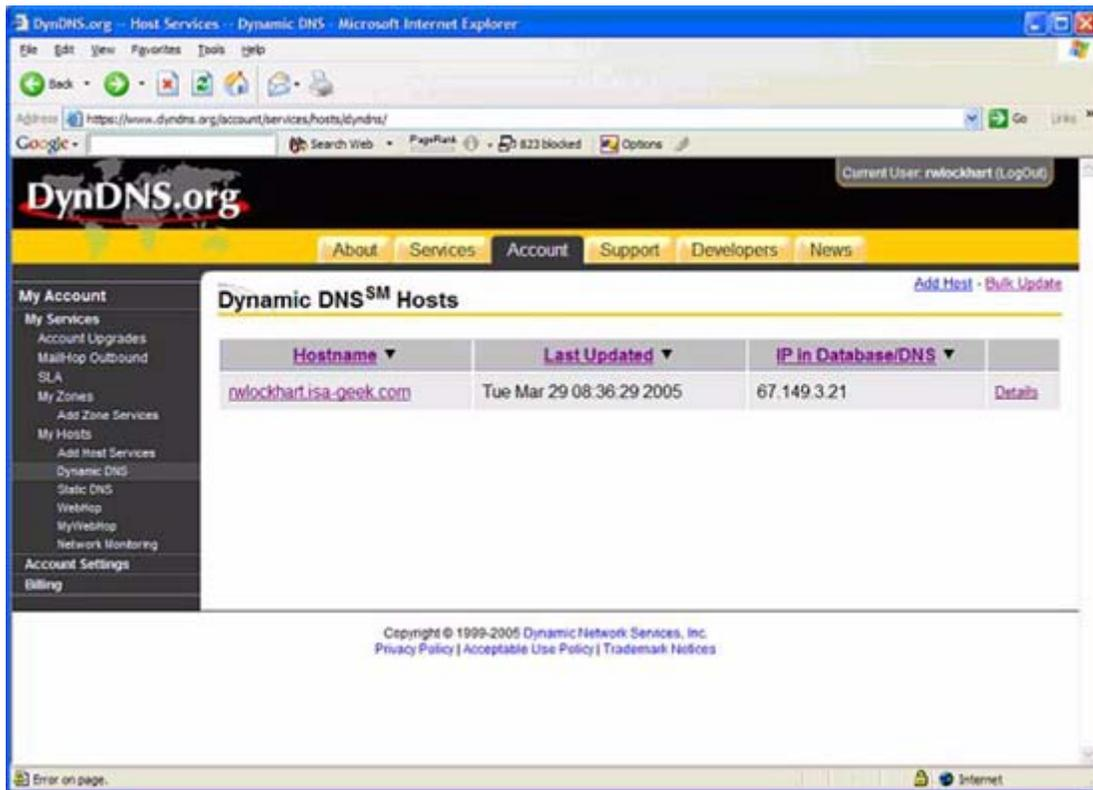
**Figure #3** – A screenshot from the DDNS website www.dyndns.com. After logging in it's easy to determine the public IP address of any router exposed to the Internet.
