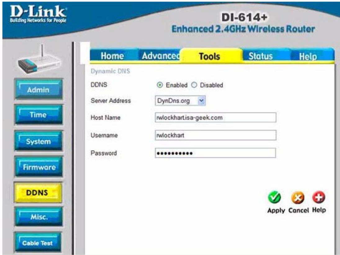
**Figure #2** – Screen shot of the DDNS configuration panel for a D-link wireless router.
