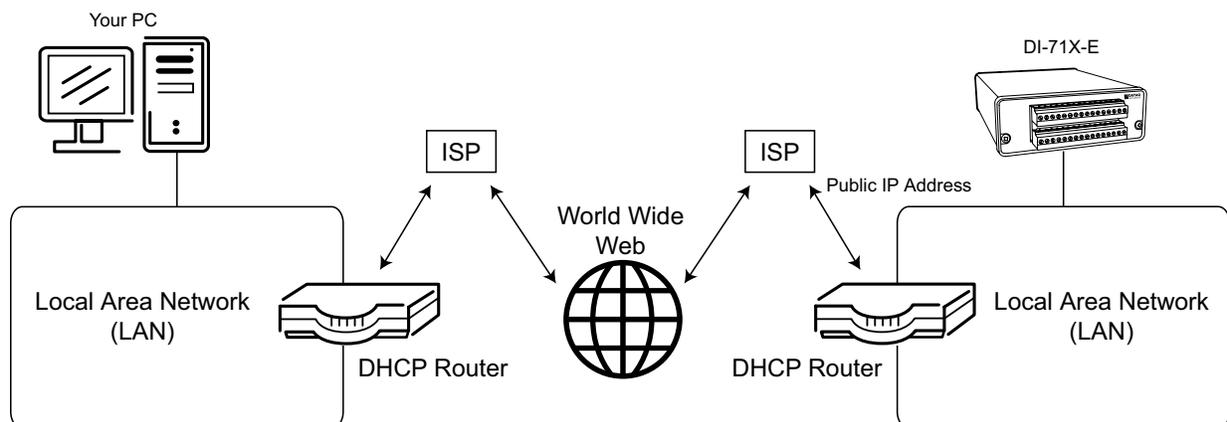
**Figure #1** -- Properly Managed, any DI-71X device can be accessed from any location in the world through the internet.
