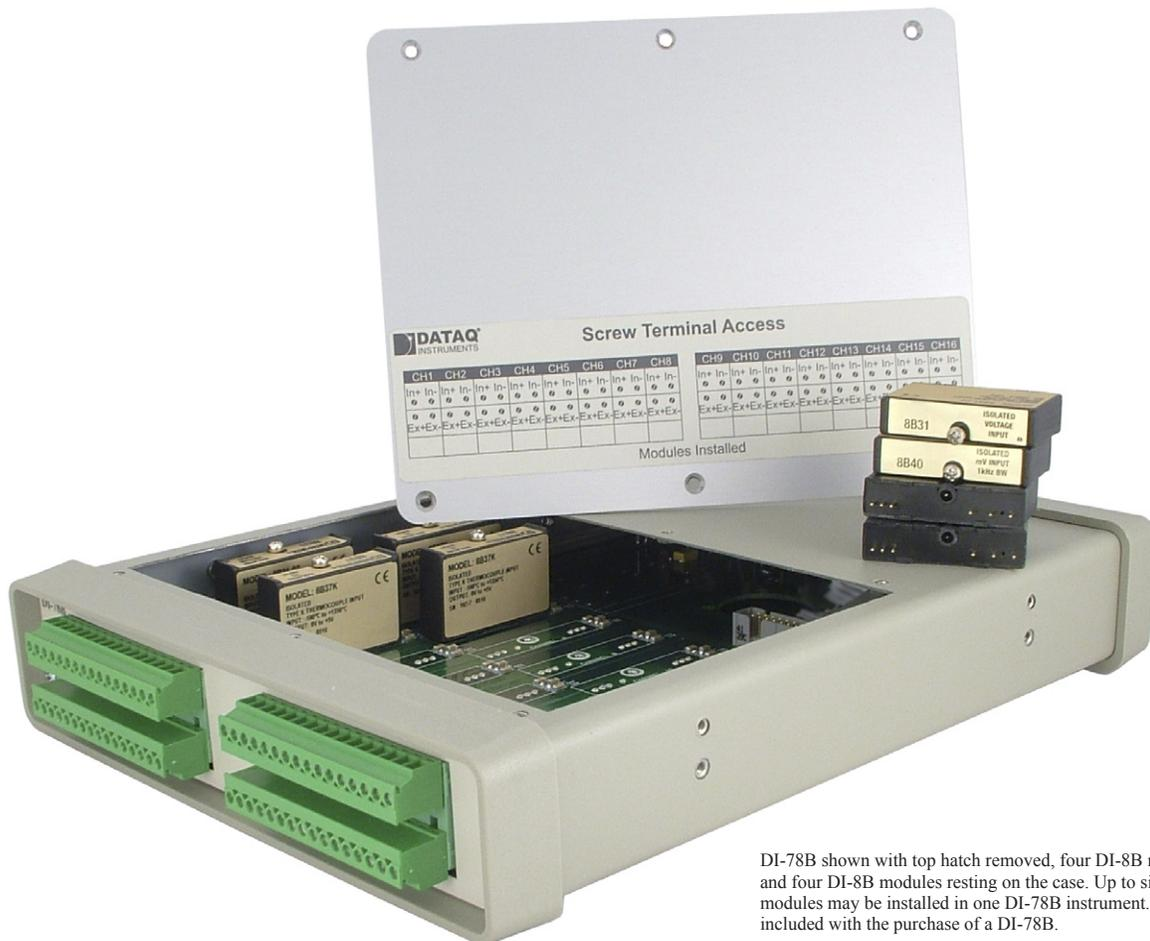
DI-78B shown with top hatch removed, four DI-8B modules installed, and four DI-8B modules resting on the case. Up to sixteen DI-8B modules may be installed in one DI-78B instrument. Modules are NOT included with the purchase of a DI-78B.
