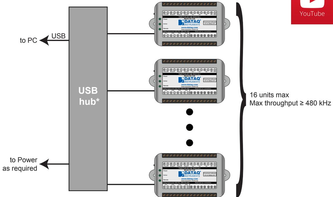
\*DATAQ Instruments 7-port USB hub (part number 2000310). Cascade for a higher port count.
