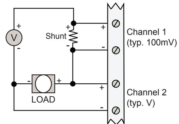
\*Model R250, 250 shunt resistor, see Ordering Guide
