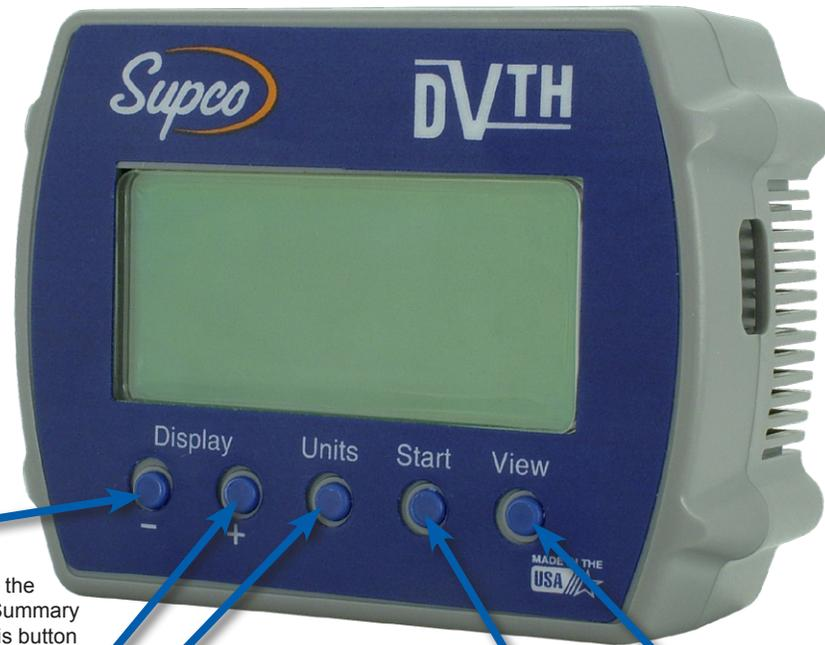
**Display -:** Use this button to decrease the screen contrast when in Sample and Summary screens. When in the Graph screen this button shifts the graph to the left, allowing you to scan backward in time to earlier-acquired data.
